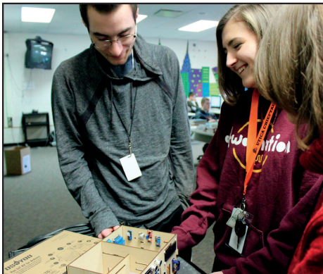
Internet of Things (IoT) Smart Home Kit enables seniors Nicholas Mitchell and Alexa Reynolds to have a hands-on smart home system experience. Labs include Wifi programming & control. Labs include monitoring and controlling home temperature and humidity in a web browser; controlling a servo motor and turning on an LED with a smart phone.
